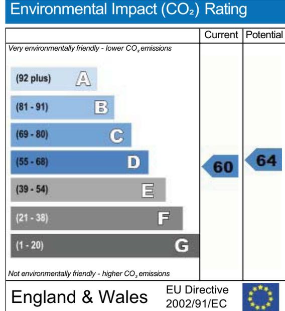
The environmental impact rating is a measure of a home's impact on the environment in terms of carbon dioxide (CO<sub>2</sub>) emissions. The higher the rating, the less impact it has on the environment.
