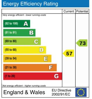
The energy efficiency rating is a measure of the overall efficiency of a home. The higher the rating, the more energy efficient the home is and the lower the fuel bills will be.
